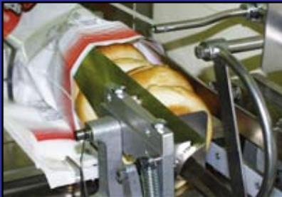
After the product is placed in the bag, the bag openers release and product motion separates the bag from the wicket.
