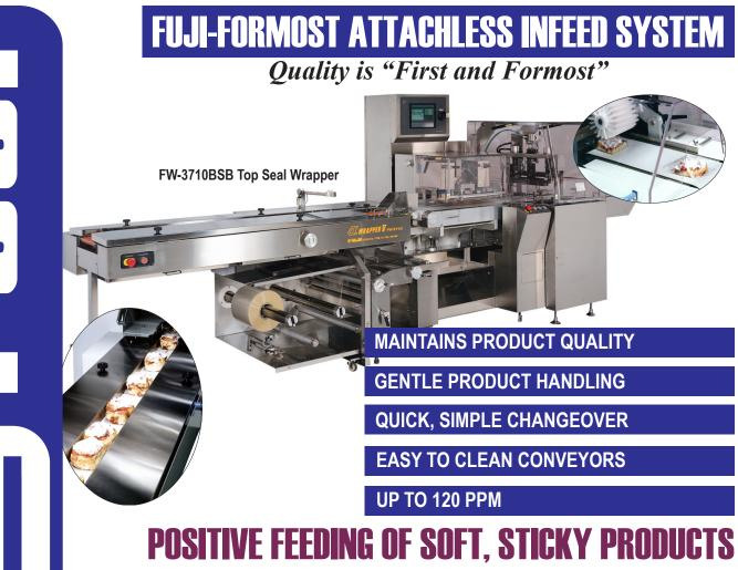
The Fuji-Formost Attachless Infeed System is specially designed to handle soft or sticky products that are impossible to wrap with lug chain systems. A flat conveyor belt transfers the product to the wrapper. The belt can be easily cleaned and removed.
