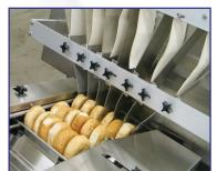
of a metering conveyor, shaker table, laning conveyor, grouper, drop chute, and rotary indexer. The unit deposits counted and stacked bagels into a Formost bagger bucket infeed conveyor.
