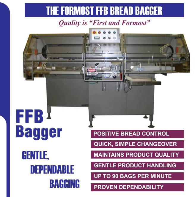
Bread feeds directly from your flighted conveyor or slicer into the Formost Fuji FFB Bagger. The unit can also provide one person operation for unsliced bread or products in trays. Specially designed paddles move the loaf into the bag with a gentle hand-like motion. Our innovative bag opening system is available optionally to provide for greater tolerance of irregularities.
