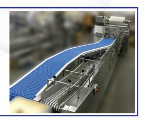
With a complete inline flow design, the Bun System eliminates problems with 90 degree transfers and provides for a more efficient and simple floorplan.
