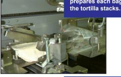
After the tortillas are placed in the bag, the bag openers release and the belt discharge conveyor moves the bag out of the bagger.
